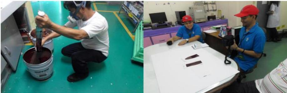
EMB personnel test for lead in paint samples using X-ray fluorescence (XRF) on 5 February 2016. [Nippon Paint]
