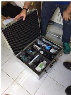
**Figure 10** Set of gold amalgam manual mercury samplers donated by the Ministry of the Environment of Japan [EMB]
