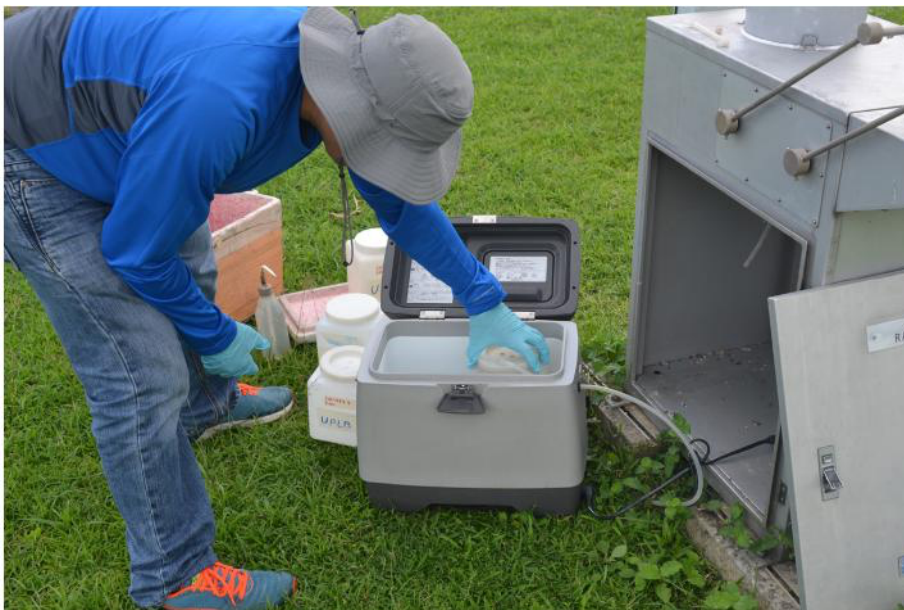
An EMB technical staff collects a wet deposition sample at the monitoring site in the University of the Philippines Los Baños in 2016. Samples are collected weekly. [EMB]
